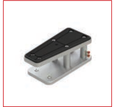
Custom fixture for making trapezoidal parts
