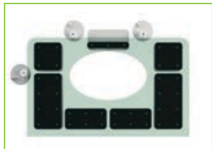
Three stops are needed to locate a part
