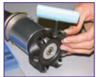
Installing Carbide Inserts (left-handed thread)
